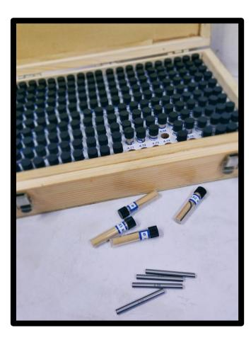
Measuring pins are used to measure ID of hole. Multi gauging.
